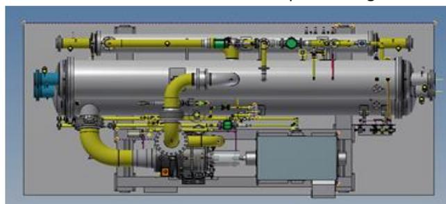
water already used to heat the district heating network. This configuration increases the amount of heat recovered from the geothermal water and maximizes heat pump performance. The district heating water leaving the geothermal heat exchangers with up to 72°C flows through the condensers of the heat pumps and is leaving them at up to 88°C. Thus, the innovative system feeds 27,000 MWh of renewable energy in the district heating network.
