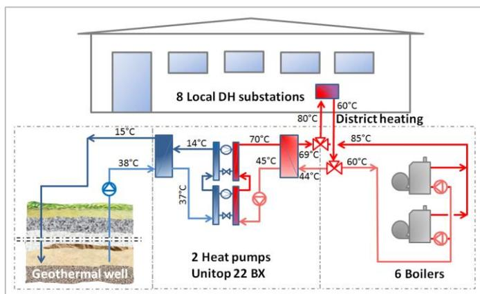
The Loup Pendu - district heating station of Plessis-Robinson draws the energy needed through two closed loop wells from the Neocomian aquifer at a depth of 850m. The supply well is located next to the machine room. Hydro-cyclonic filters remove sand and other solid matter with very little head loss. The reinjection well is located 900m downstream of the supply well.
